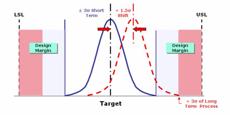
The Short Term distribution is "shifted" +1.5 $\sigma$  to simulate the +3 $\sigma$  value of the long term process distribution
