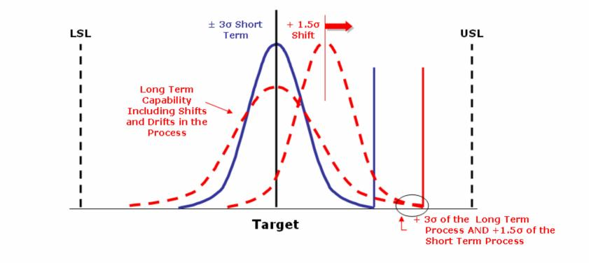
The +3 $\sigma$  value of the long term distribution has the same tail area probability for a defect as the +1.5 $\sigma$  "shifted" short term distribution.
